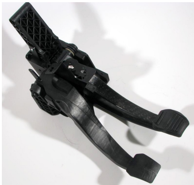
Fig. 1 Pedal box with all-plastic clutch pedal and brake pedal in polyamide composite sheet hybrid technology
