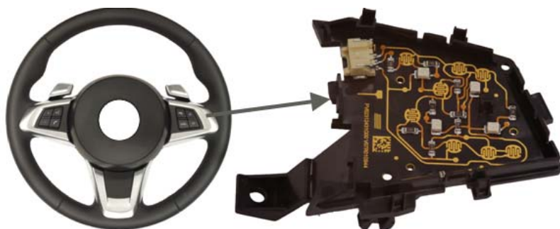
Fig. 1 Steering wheel with right and left steering wheel control switch
